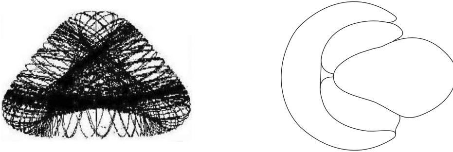
Figure 14.1 Henon-Heiles Attractor: (Left) Phase Portrait and (Right) Corresponding Poincaré Section
